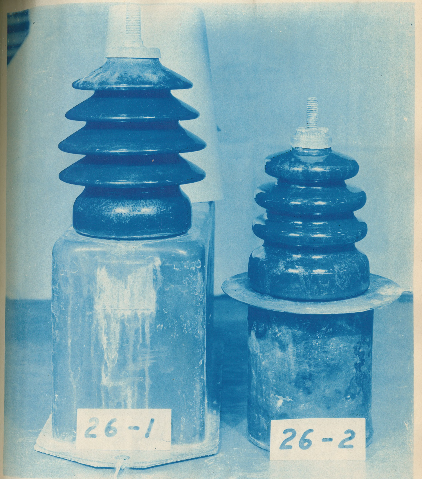
(A) OVERSIZE 5KV PORCELAIN BUSHING (B) STANDARD 5KV PORCELAIN BUSHING
